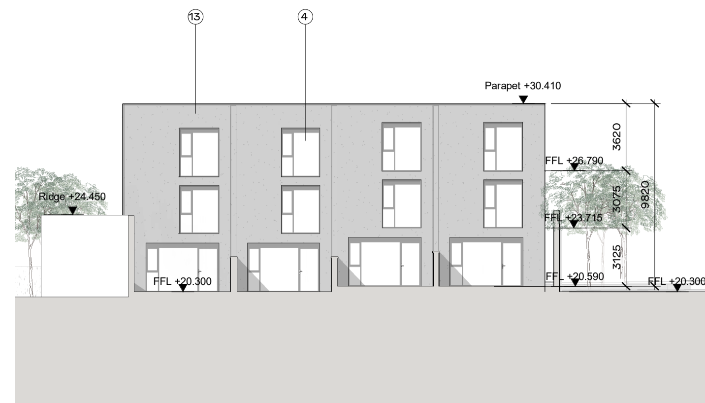
1 Block Elevation BG5 West Elevation 1 : 200
